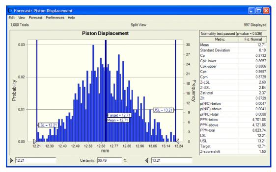
Figure 186 Piston Displacement Forecast Chart
