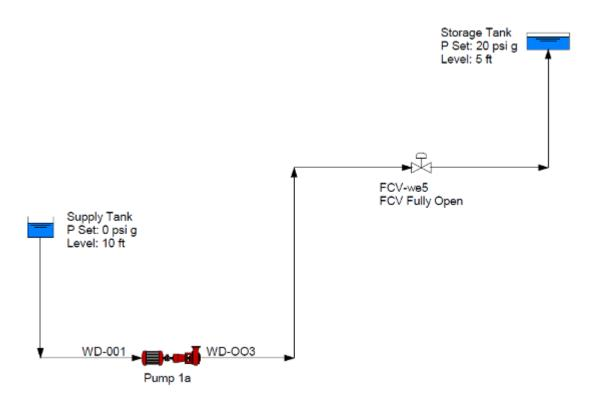
Let's say you want to see how long it will take Pump 1a to lower the tank level in the Supply Tank from 10 ft to 5 ft. This is a time simulation type of problem. As the Supply Tank is pumped down the Storage Tank is filled. This change in elevation of both the Supply and Storage tanks causes the static head to increase. This increase in static head causes the pump to run back on its curve resulting in a reduced flow rate through the pump as the Supply Tank is pumped down.
