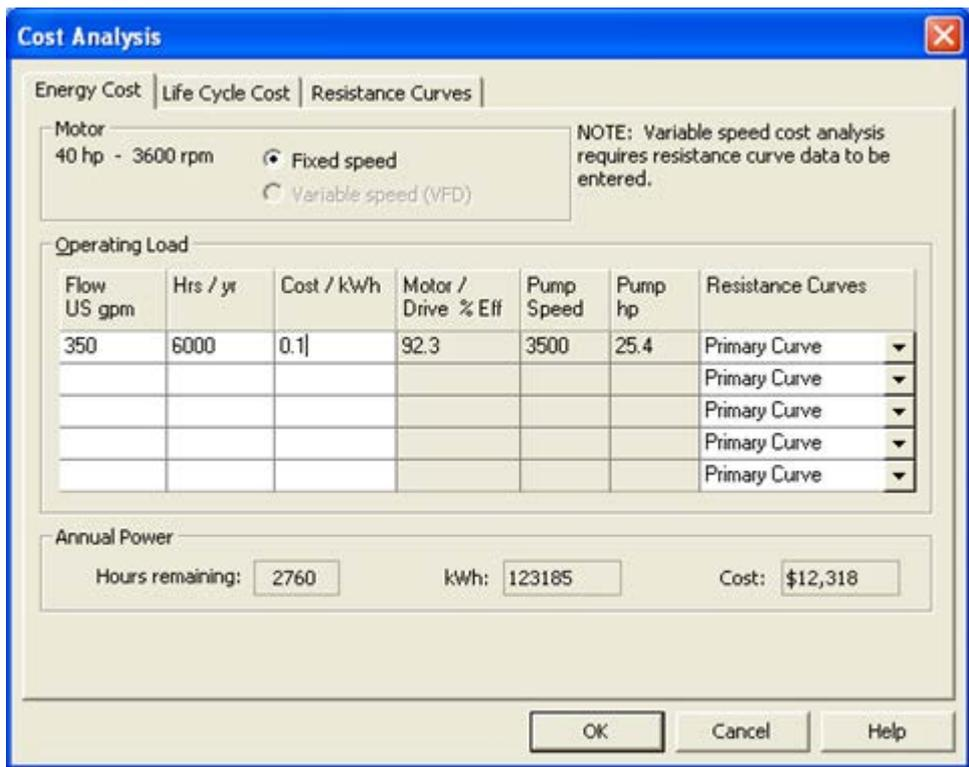
Notice the operating cost for PUMP 124a with the smaller impeller diameter is \$12,318, or a savings of over \$7,200 per year!
