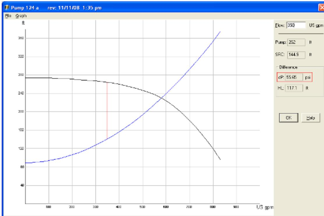
Notice the difference in pressure between the pump curve and the system curve is over 55 psi. This difference must be made up at the control valve. Our selected globe valve must drop even more (over 61 psi) to limit the flow to 350 gpm.
